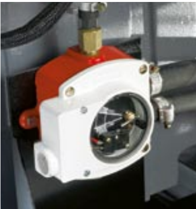
Automatic oil filler extending the service intervals
